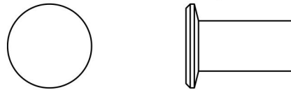
Flat Top Countersunk Head (With Chamfered Top)
