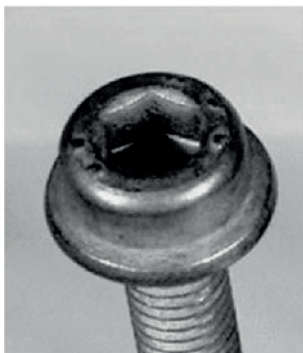
a) Zinc-nickel after 72 h NSS testing
