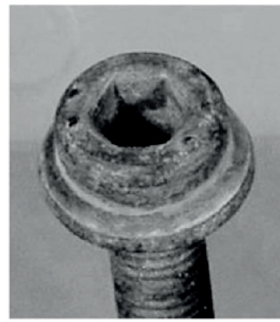
b) Zinc-nickel after 1 000 h NSS testing
